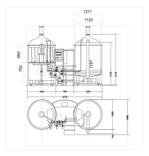
This boiling equipment V600 is mounted in a rigid frame made of 1.4301, 8 pc adjustable supports installed in its bottom part.
